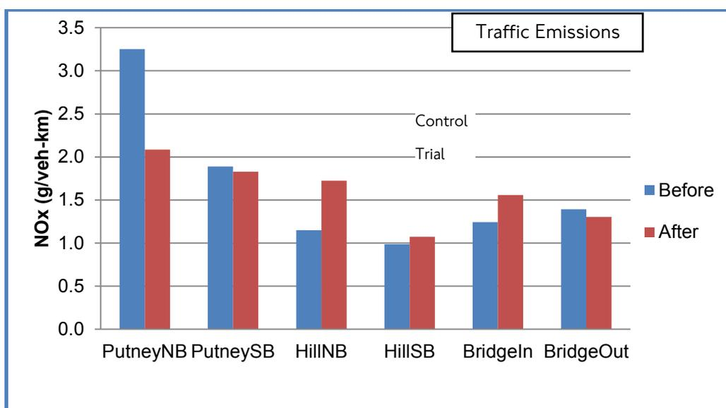
Results calculated from actual Bus trajectory data show a universal reduction in emissions in both the Protected and Enabling zones. Results from the VISSIM-PHEM model for general traffic show a clear reduction in emissions in the Protected Zone, with an increase in the Enabling Zone as expected. The model can now be used to test other strategies offline, apply fleet changes and assess the emissions impacts of proposed schemes. The method can now be repeated elsewhere with the same technology.
