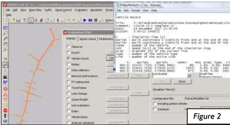
To provide comparison of vehicle emissions in both scenarios, the VISSIM data for every vehicle is exported to leading emissions modelling software PHEM. This uses the speed, gradient, position, acceleration of every simulated vehicle for every second to calculate the emissions. The accumulated data is compiled to provide a detailed picture of the impact on vehicle emissions. Figure 2 shows the VISSIM model.
